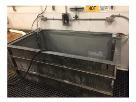
**Reason BHC Won:** 3887 GD provided better cleaning results with no foaming issues. BHC & the distributor provided "Tank Titration" Support and recommended they replace "Air" agitation with "Eductor Spray System to reduce foaming
