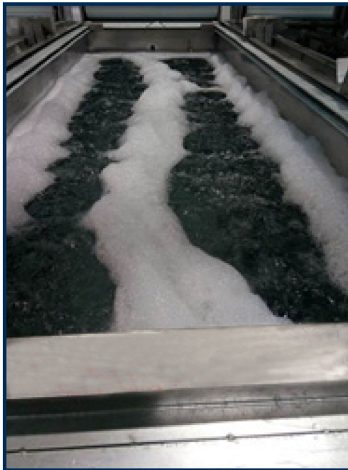
Figure 2: Drag out of detergent into Rinse 1
