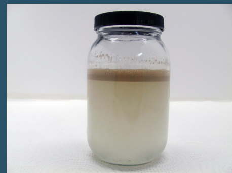
Oil layer (on top) Clean solution for reuse (below)
