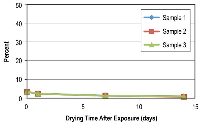
Figure 64. Weight gain of PTFE after 60 days in Solstice PF.
