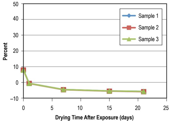
Figure 74. Weight gain (loss) of Buna N (NBR) after 90 days in L-14780.
