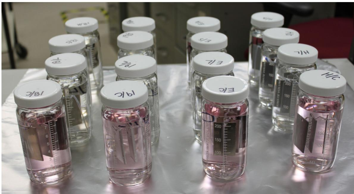
Figure 1. Metal specimens immersed in four test solvents at beginning of exposure.
