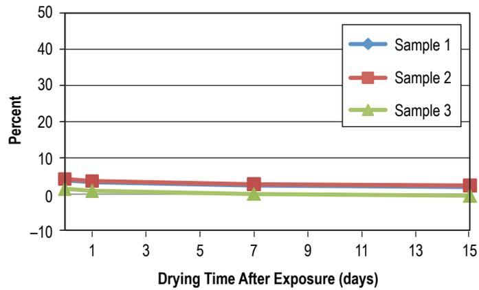
Figure 53. Weight gain of PTFE after 90 days in AK-225G.
