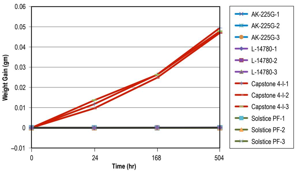
Figure 23. Weight gain or loss over time of 17-4PH stainless steel after immersion in four solvents.
