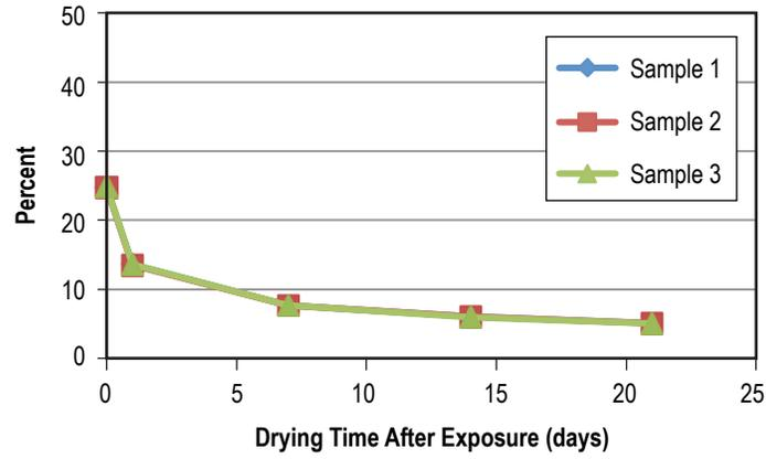
Figure 69. Weight gain of FKM V0747-75 after 30 days in L-14780.
