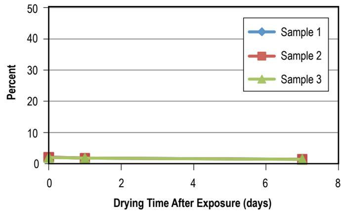
Figure 92. Weight gain of PTFE after 90 days in Solvokane.
