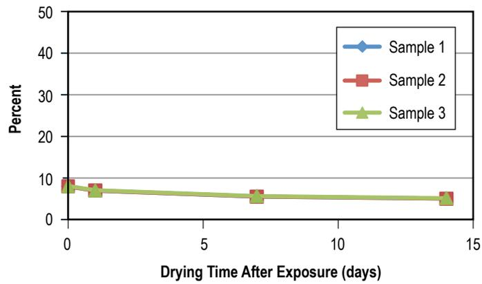
Figure 103. Weight gain of PTFE after 60 days in Capstone 4-I.
