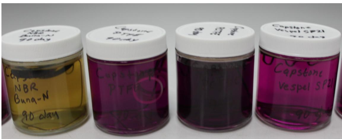
Figure 30. Capstone 4-I after nonmetal immersion for 90 days.
