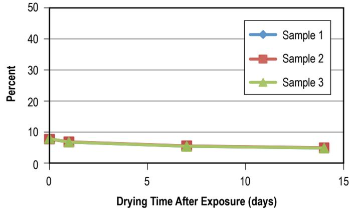
Figure 102. Weight gain of PTFE after 30 days in Capstone 4-I.
