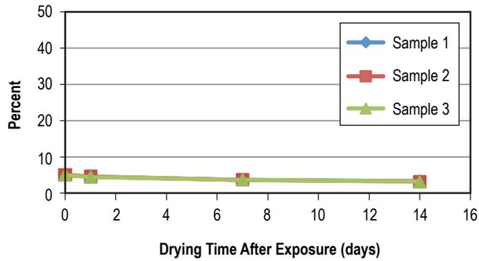
Figure 52. Weight gain of PTFE after 60 days in AK-225G.
