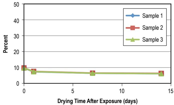
Figure 56. Weight gain of PCTFE after 90 days in AK-225G.
