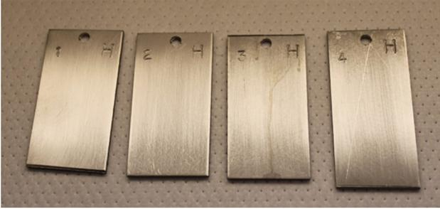
Figure 3. Stainless steel after 21 days in AK-225G.
