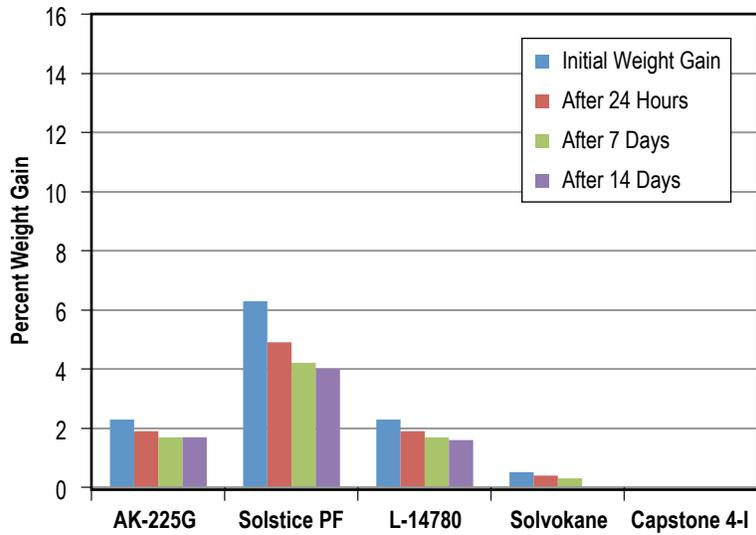
Figure 114. Weight gain of Kel-F PCTFE retained after 30-day immersion in five solvents.
