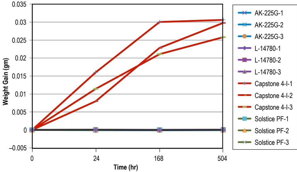
Figure 25. Weight gain over time of 2219-T6 aluminum after immersion in four solvents.
