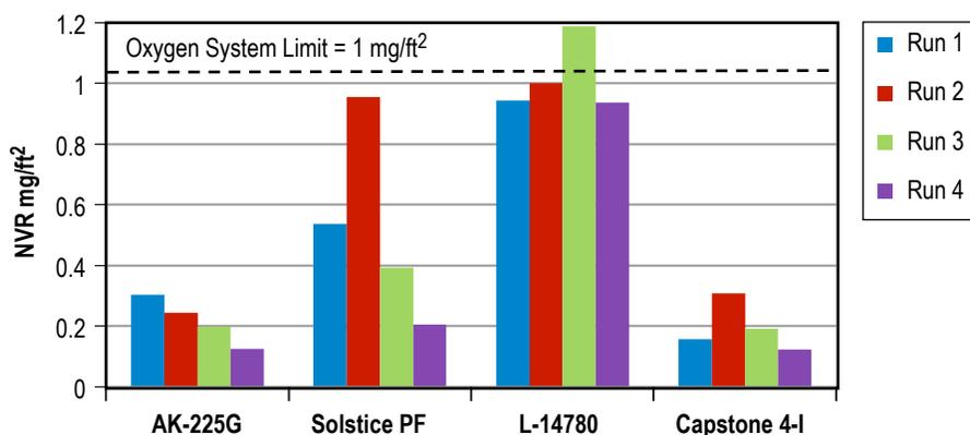
Figure 40. NVR level achieved as measured by rinsing with AK-225G.
