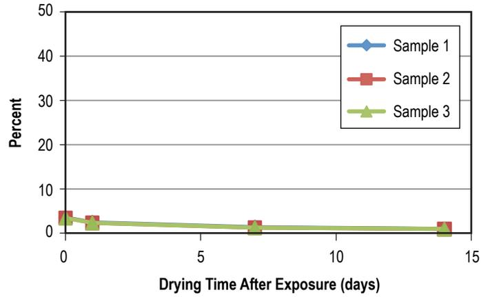
Figure 63. Weight gain of PTFE after 30 days in Solstice.
