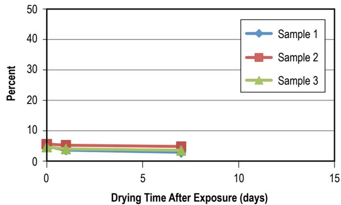
Figure 80. Weight gain of PCTFE after 90 days in L-14780.
