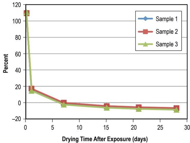
Figure 50. Weight gain (loss) of Buna N (NBR) after 90 days in AK-225G.
