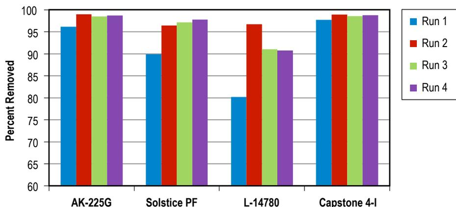
Figure 39. Field cleaning—comparison of tube cleaning efficiencies.
