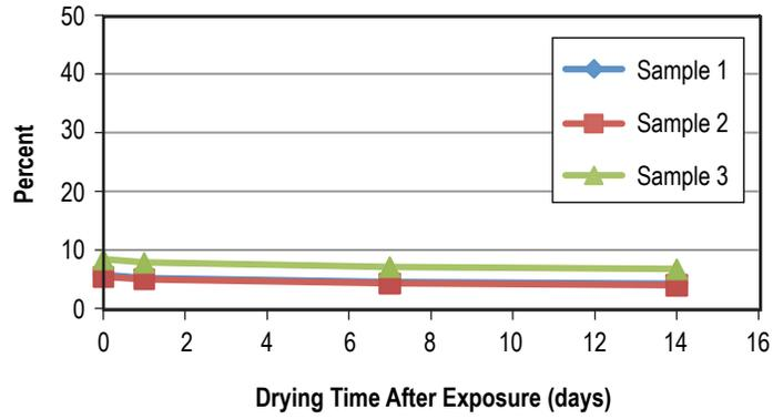
Figure 51. Weight gain of PTFE after 30 days in AK-225G.
