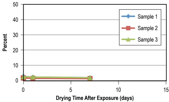
Figure 94. Weight gain of Vespel SP21 after 60 days in Solvokane.
