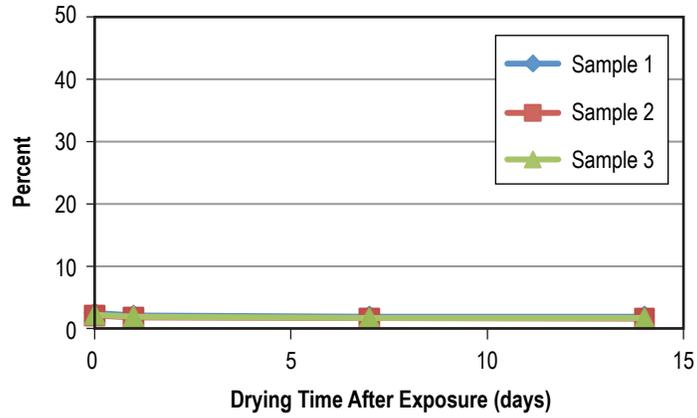
Figure 54. Weight gain of PCTFE after 30 days in AK-225G.
