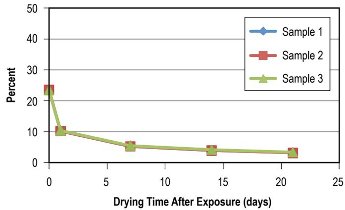
Figure 85. Weight gain of FKM V0747-75 after 60 days in Solvokane.
