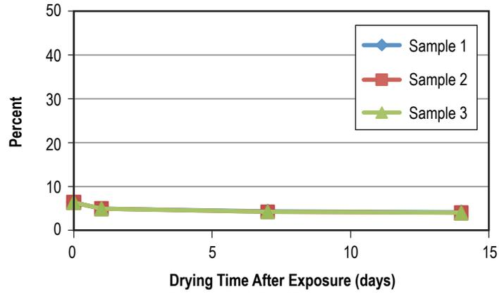
Figure 66. Weight gain of PCTFE after 30 days in Solstice PF.
