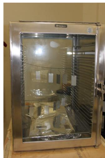
Figure 32. Coupons in desiccator.
