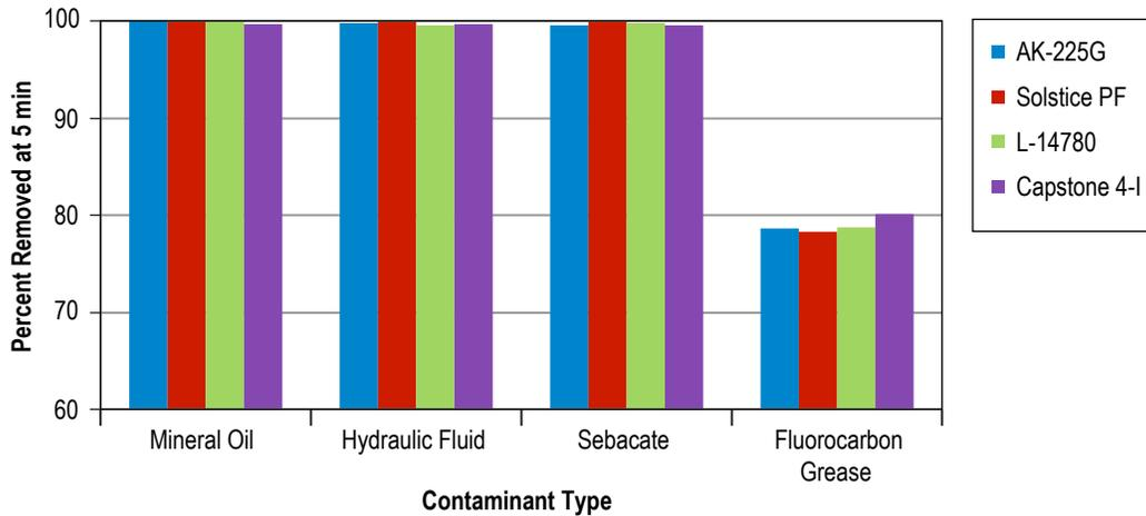
Figure 36. Comparison of contaminant removal effectiveness by static immersion.
