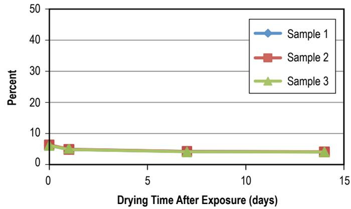
Figure 68. Weight gain of PCTFE after 90 days in Solstice PF.
