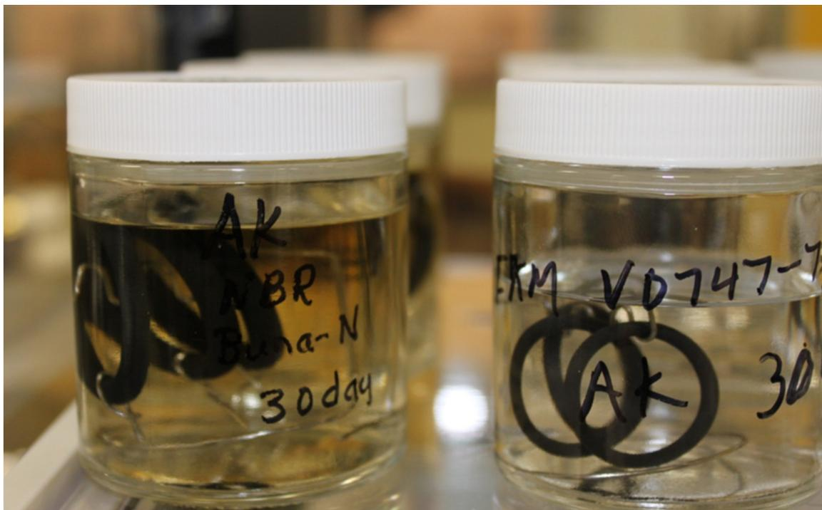
Figure 29. O-ring specimens immersed in solvent with stainless steel wire supports.
