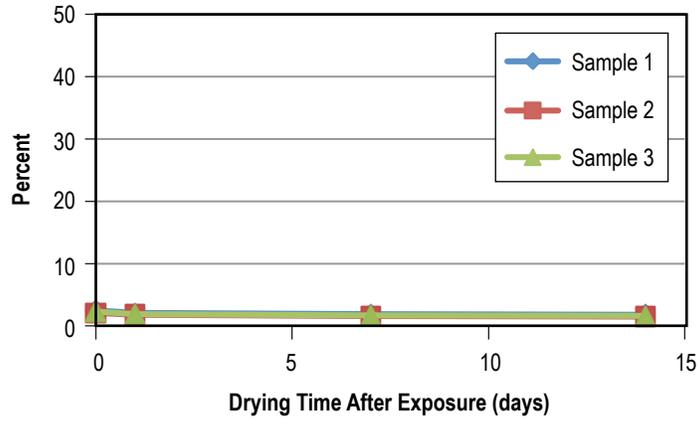
Figure 78. Weight gain of PCTFE after 30 days in L-14780.
