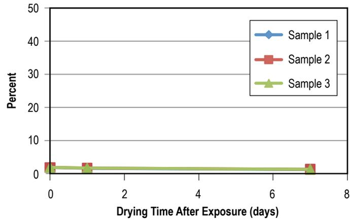
Figure 91. Weight gain of PTFE after 60 days in Solvokane.
