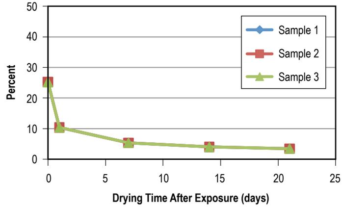
Figure 84. Weight gain of FKM V0747-75 after 30 days in Solvokane.
