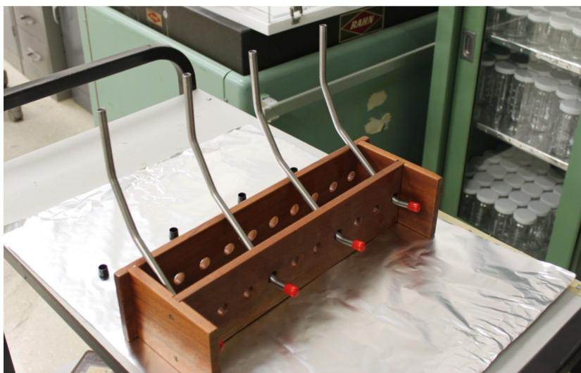
Figure 37. Stainless steel tubes with end caps used for the field cleaning test.
