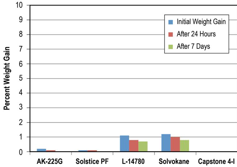
Figure 121. Weight gain of PEEK retained after 60-day immersion in five solvents.
