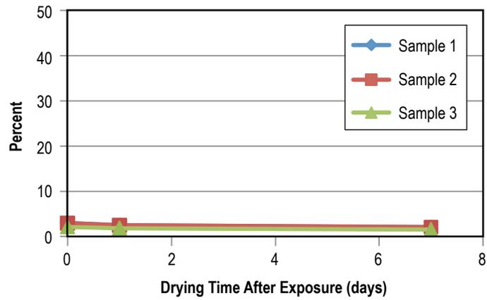
Figure 82. Weight gain of Vespel SP-21 after 60 days in L-14780.
