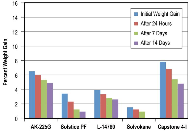
Figure 111. Weight gain of PTFE retained after 30-day immersion in five solvents.
