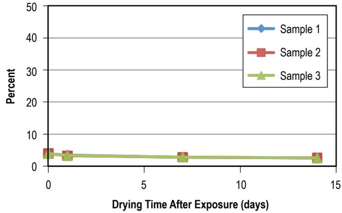
Figure 75. Weight gain of PTFE after 30 days in L-14780.
