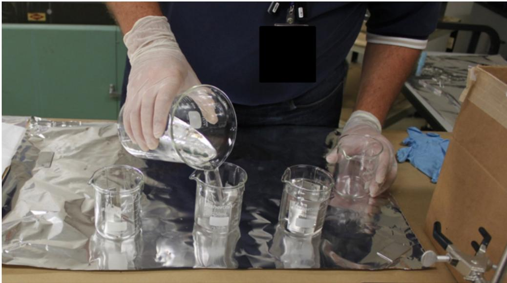
Figure 35. Addition of test solvent to beakers containing suspended coupons.
