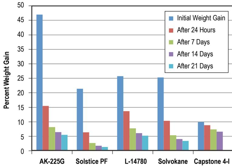
Figure 105. Weight gain of FKM V0747-75 retained after 30-day immersion in five solvents.
