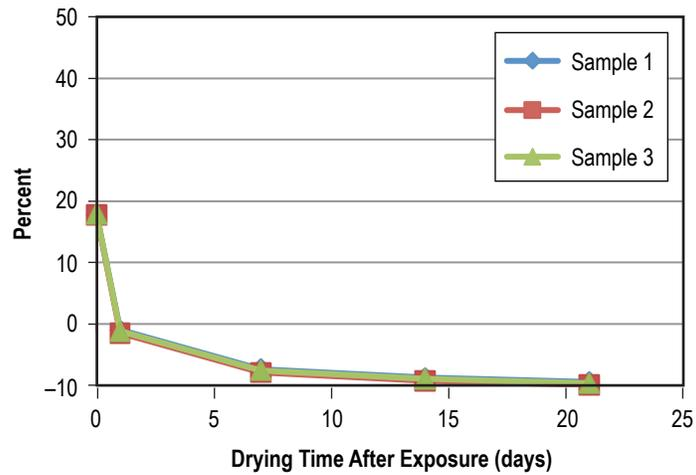
Figure 61. Weight gain (loss) of Buna N (NBR) after 60 days in Solstice PF.
