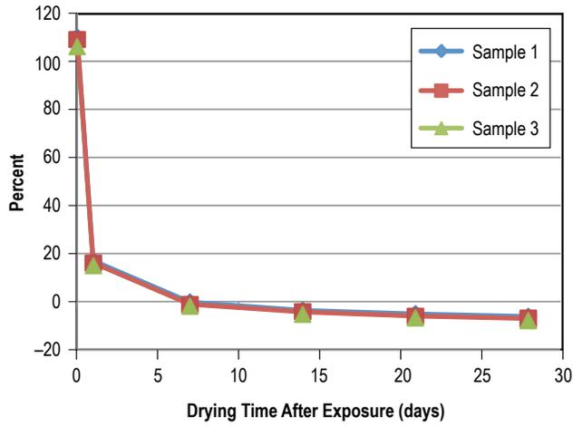
Figure 48. Weight gain (loss) of Buna N (NBR) after 30 days in AK-225G.
