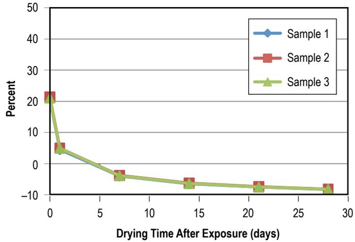
Figure 87. Weight gain (loss) of Buna N (NBR) after 30 days in Solvokane.
