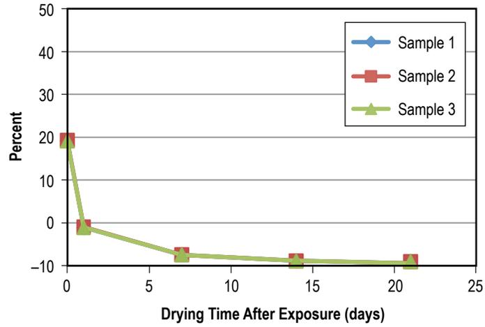
Figure 60. Weight gain (loss) of Buna N (NBR) after 30 days in Solstice PF.
