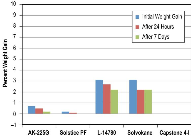
Figure 119. Weight gain of Vespel SP-21 retained after 90-day immersion in five solvents.
