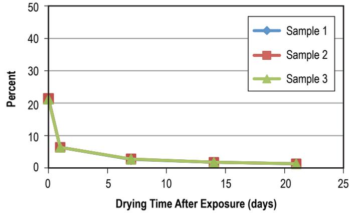
Figure 57. Weight gain of FKM V0747-75 after 30 days in Solstice PF.
