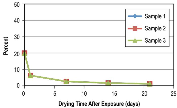
Figure 58. Weight gain of FKM V0747-75 after 60 days in Solstice PF.
