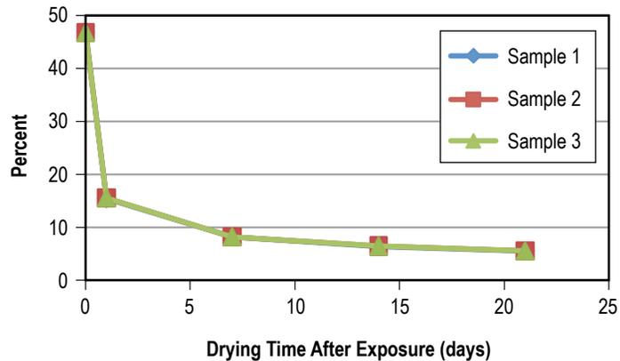
Figure 45. Weight gain of FKM V0747-75 after 30 days in AK-225G.
