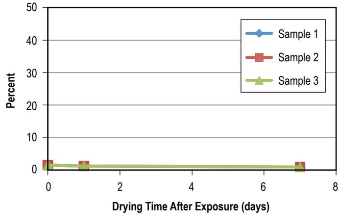
Figure 90. Weight gain of PTFE after 30 days in Solvokane.
