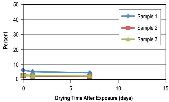
Figure 79. Weight gain of PCTFE after 60 days in L-14780.
