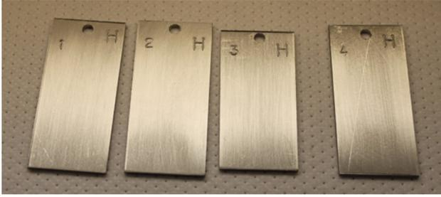
Figure 11. Stainless steel after 21 days in L-14780.
