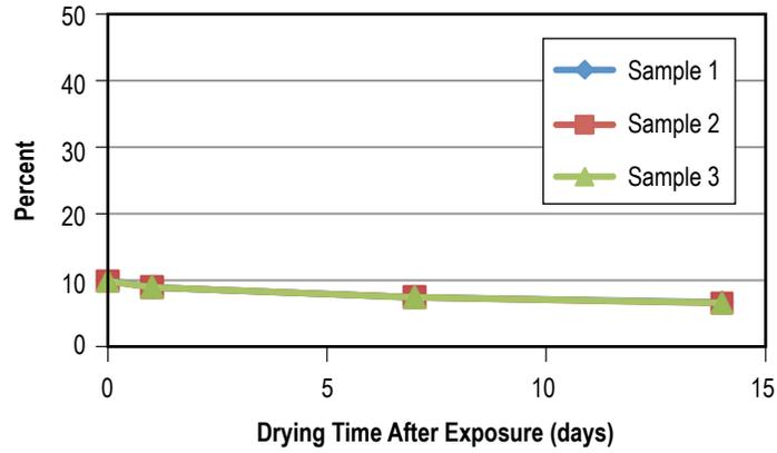
Figure 96. Weight gain of FKM V0747-75 after 30 days in Capstone 4-I.
