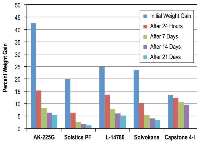
Figure 106. Weight gain of FKM V0747-75 retained after 60-day immersion in five solvents.
