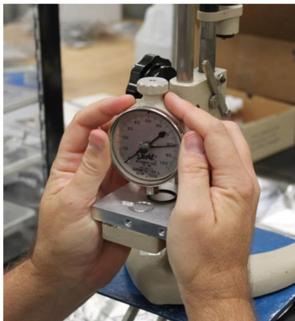
Figure 28. Measurement of Shore A durometer.
