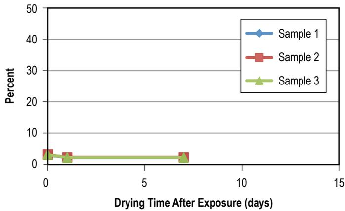
Figure 95. Weight gain of Vespel SP21 after 90 days in Solvokane.
