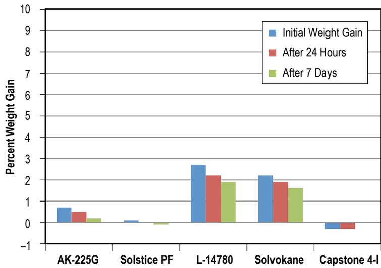
Figure 118. Weight gain (loss) of Vespel SP-21 retained after 60-day immersion in five solvents.
