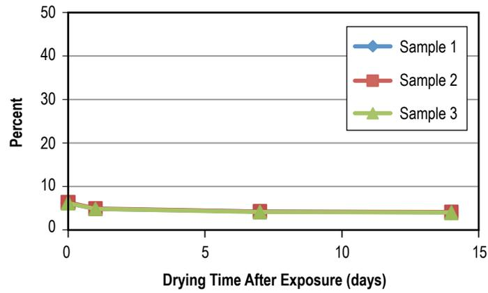
Figure 67. Weight gain of PCTFE after 60 days in Solstice PF.
