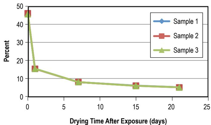
Figure 47. Weight gain of FKM V0747-75 after 90 days in AK-225G.
