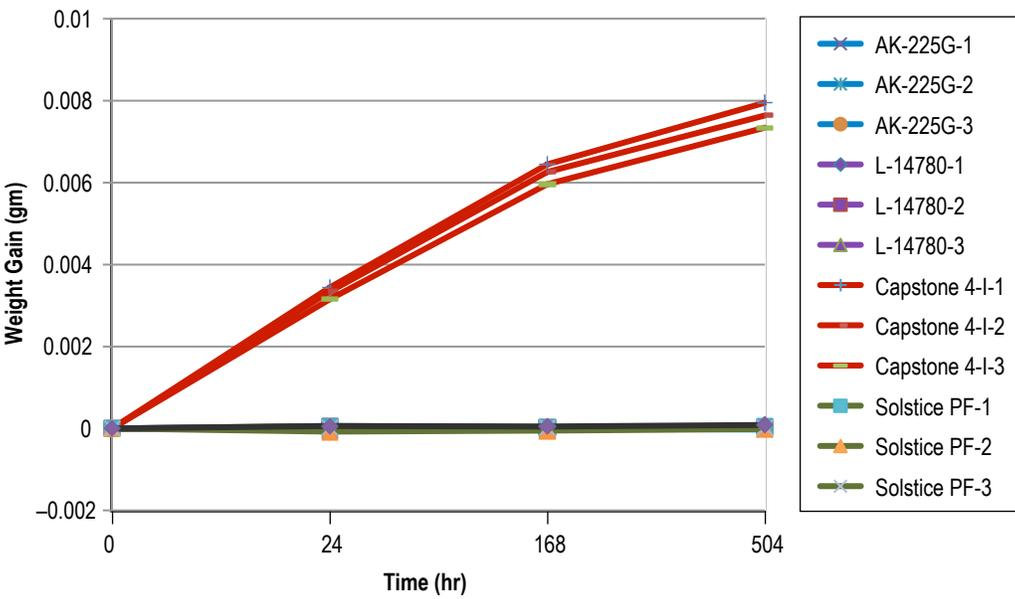
Figure 26. Weight gain or loss over time of Inconel 718 after immersion in four solvents.
