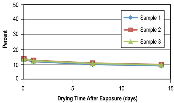
Figure 97. Weight gain of FKM V0747-75 after 60 days in Capstone 4-I.
