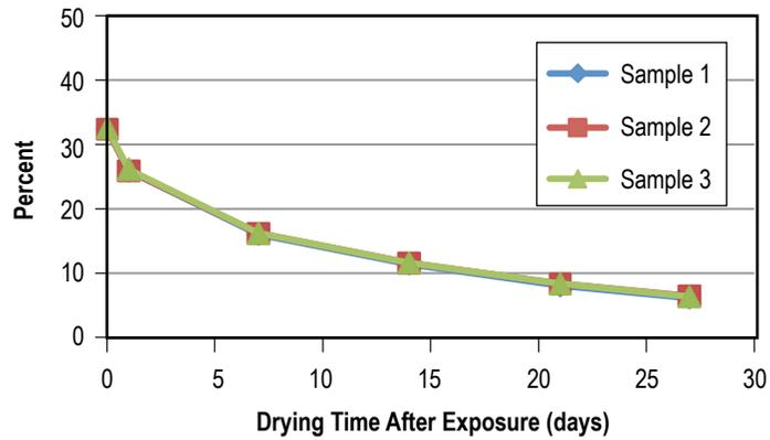
Figure 100. Weight gain of Buna N (NBR) after 60 days in Capstone 4-I.
