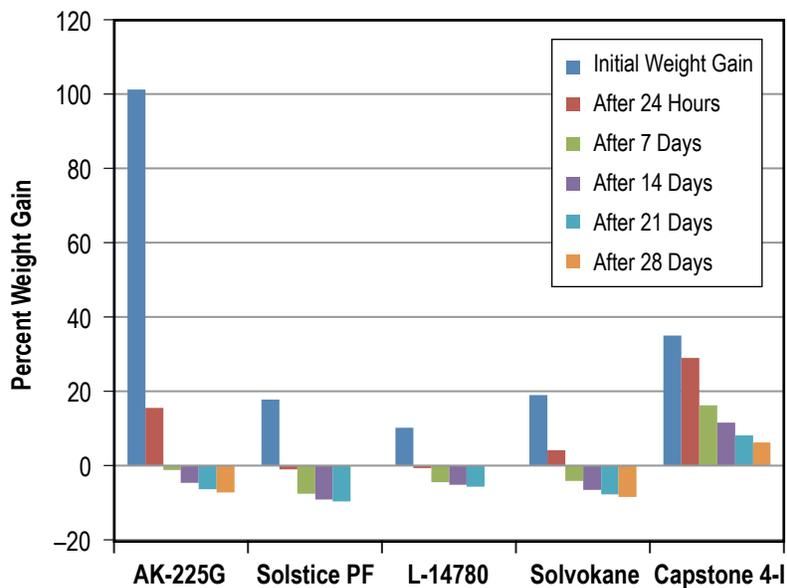
Figure 109. Weight gain (loss) of Buna N (NBR) retained after 60-day immersion in five solvents.
