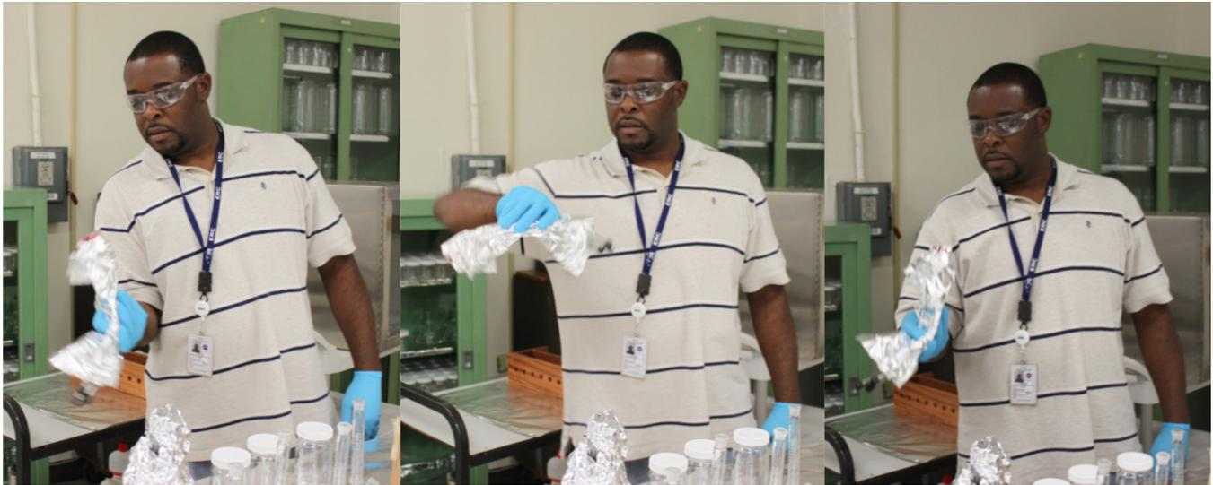
Figure 38. Rocking motion used to clean tubes simultaneously for the field cleaning test.
