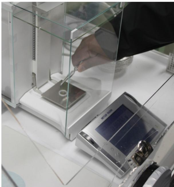
Figure 27. Weighing specimen on an analytical balance.
