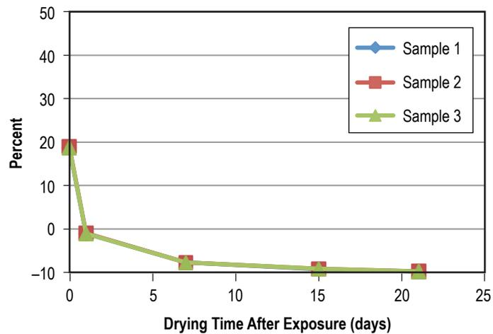
Figure 62. Weight gain (loss) of Buna N (NBR) after 90 days in Solstice PF.
