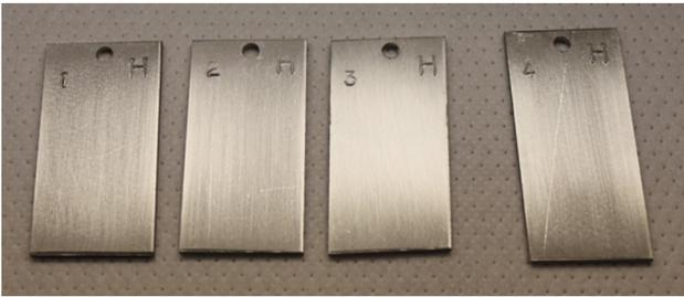
Figure 7. Stainless steel after 21 days in Solstice PF.
