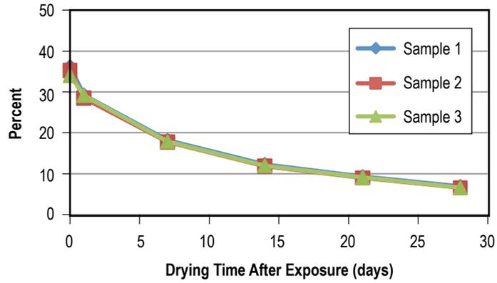
Figure 99. Weight gain of Buna N (NBR) after 30 days in Capstone 4-I.
