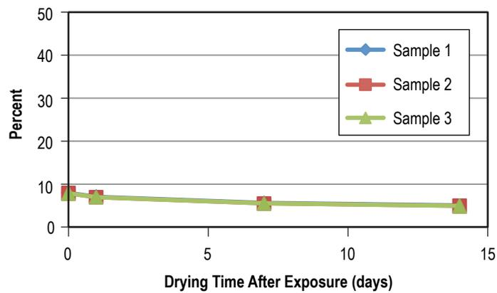
Figure 104. Weight gain of PTFE after 90 days in Capstone 4-I.
