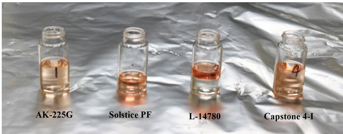
Figure 44. Contaminant mix dissolved in the test solvents showing separation in Solstice PF and L-14780.
