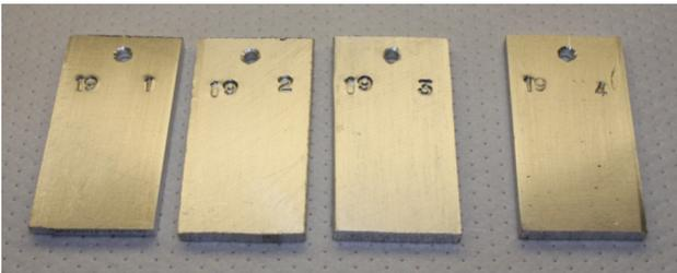
Figure 9. Aluminum after 21 days in Solstice PF.
