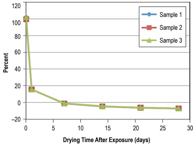
Figure 49. Weight gain (loss) of Buna N (NBR) after 60 days in AK-225G.
