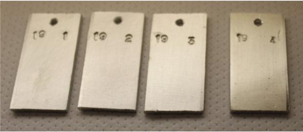
Figure 13. Aluminum after 21 days in L-14780.
