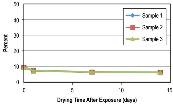
Figure 55. Weight gain of PCTFE after 60 days in AK-225G.
