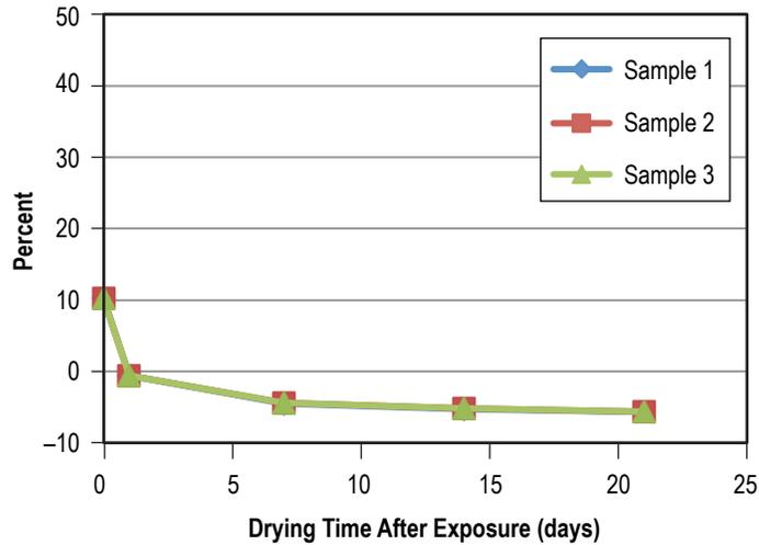
Figure 73. Weight gain (loss) of Buna N (NBR) after 60 days in L-14780.
