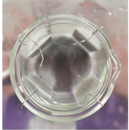
Figure 34. Coupons suspended in solvent.
