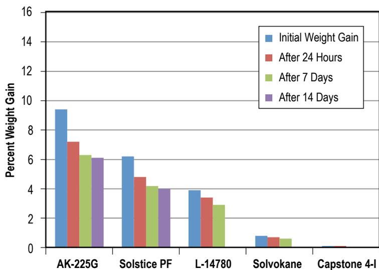
Figure 116. Weight gain of Kel-F PCTFE retained after 90-day immersion in five solvent.
