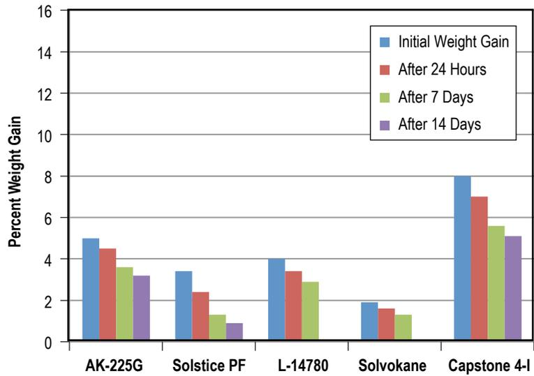
Figure 112. Weight gain of PTFE retained after 60-day immersion in five solvents.
