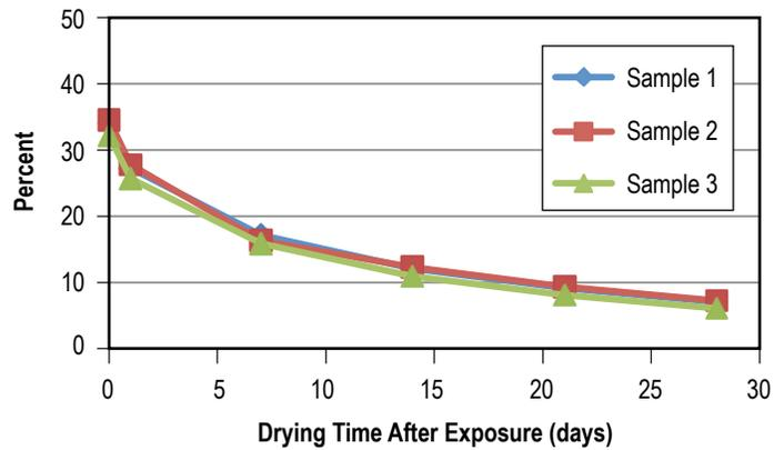
Figure 101. Weight gain of Buna N (NBR) after 90 days in Capstone 4-I.
