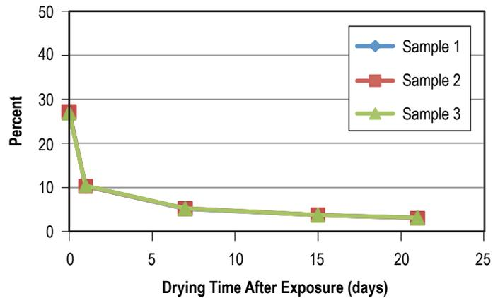
Figure 86. Weight gain of FKM V0747-75 after 90 days in Solvokane.
