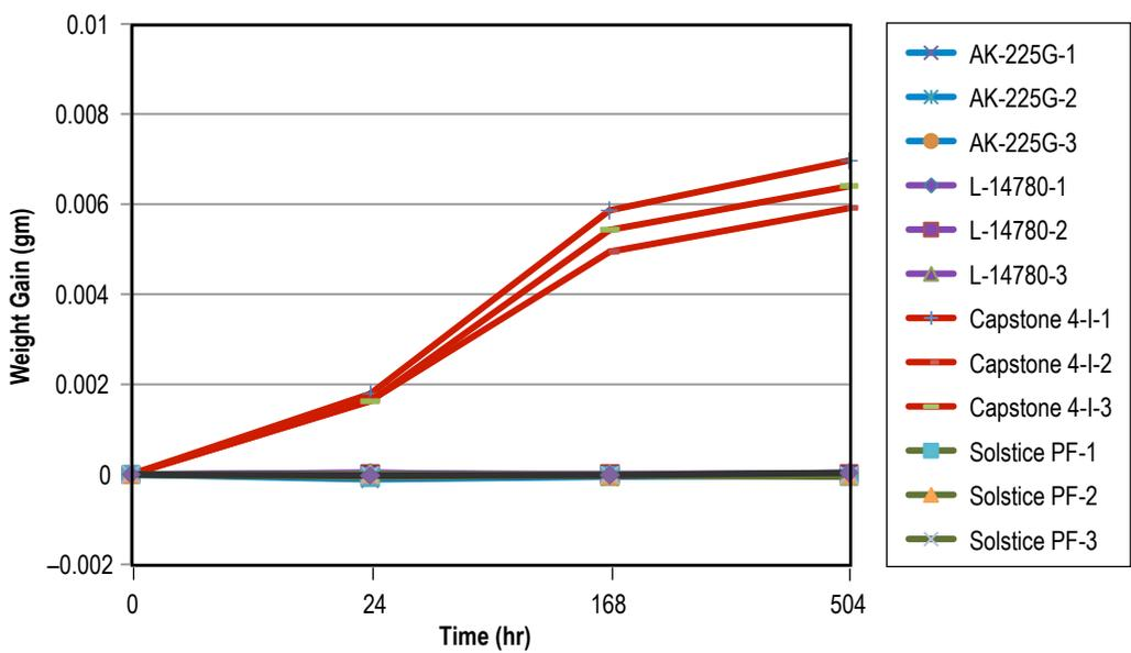
Figure 24. Weight gain over time of Elgiloy after immersion in four solvents.
