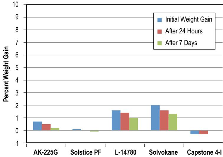
Figure 117. Weight gain (loss) of Vespel SP-21 retained after 30-day immersion in five solvents.
