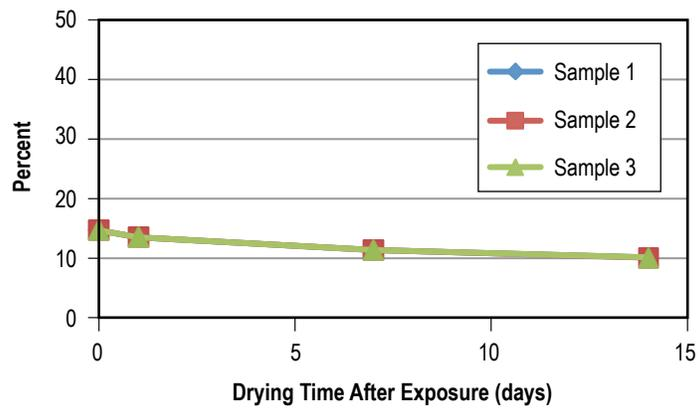
Figure 98. Weight gain of FKM V0747-75 after 90 days in Capstone 4-I.
