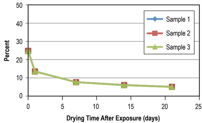
Figure 70. Weight gain of FKM V0747-75 after 60 days in L-14780.
