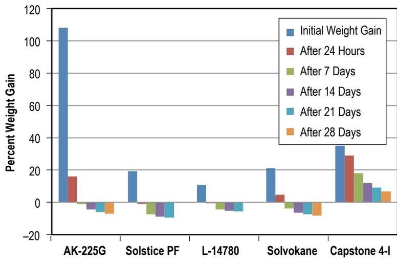
Figure 108. Weight gain (loss) of Buna N (NBR) retained after 30-day immersion in five solvents.
