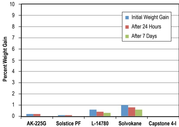
Figure 120. Weight gain of PEEK retained after 30-day immersion in five solvents.
