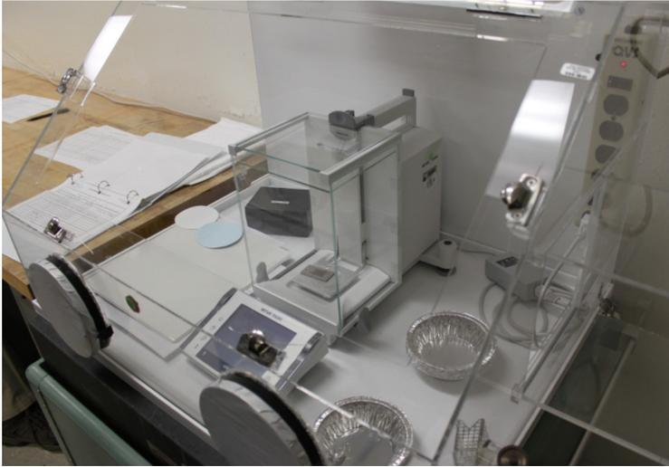
Figure 33. Analytical balance used to weigh test coupons.
