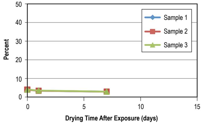
Figure 76. Weight gain of PTFE after 60 days in L-14780.
