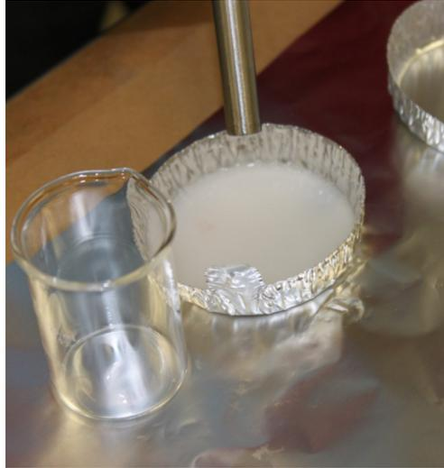
Figure 42. Milky L-14780 from tube cleaning.
