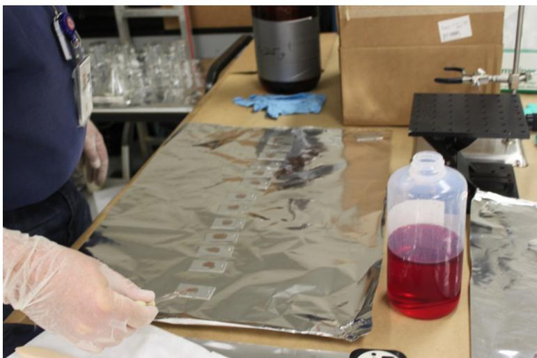
Figure 31. Application of contaminant to test coupons.
