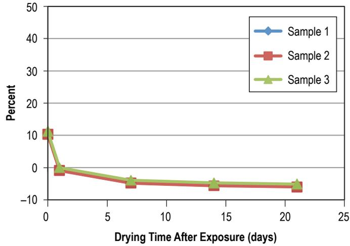
Figure 72. Weight gain (loss) of Buna N (NBR) after 30 days in L-14780.
