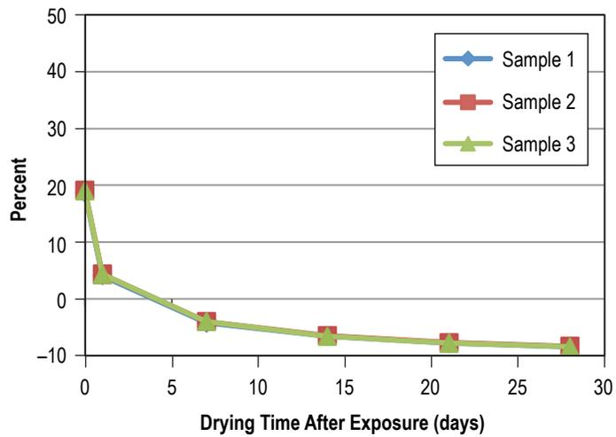
Figure 88. Weight gain (loss) of Buna N (NBR) after 60 days in Solvokane.
