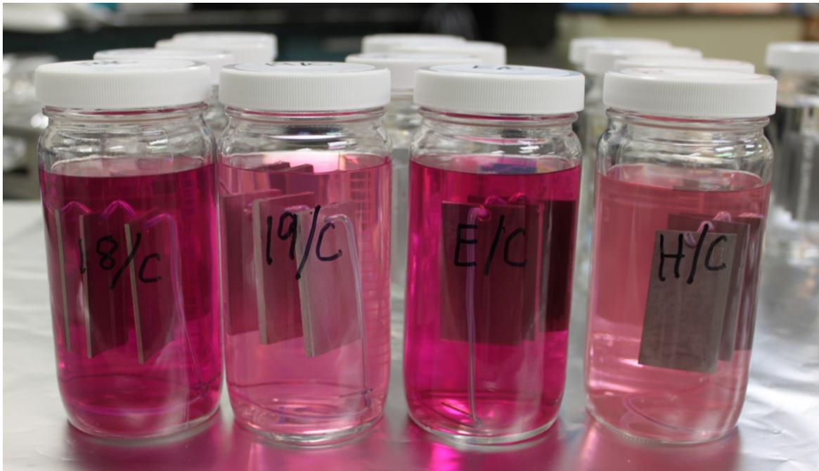
Figure 2. Metals immersed in Capstone 4-I at 24 hours.
