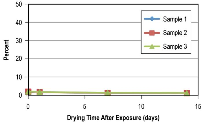
Figure 93. Weight gain of Vespel SP21 after 30 days in Solvokane.
