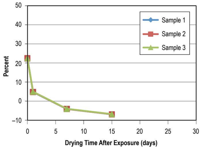
Figure 89. Weight gain (loss) of Buna N (NBR) after 90 days in Solvokane.
