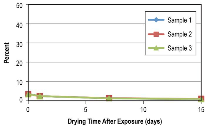
Figure 65. Weight gain of PTFE after 90 days in Solstice PF.
