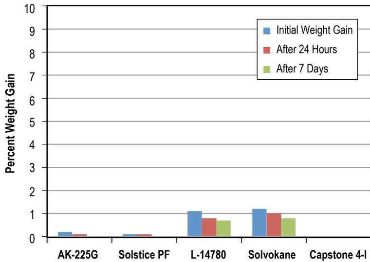
Figure 122. Weight gain of PEEK retained after 90-day immersion in five solvents.
