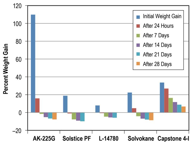
Figure 110. Weight gain (loss) of Buna N (NBR) retained after 90-day immersion in five solvents.
