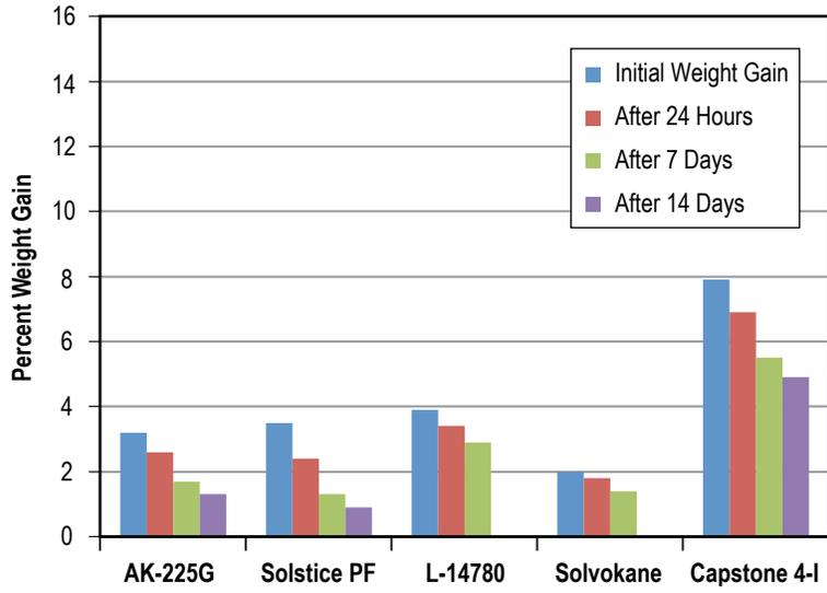
Figure 113. Weight gain of PTFE retained after 90-day immersion in five solvents.
